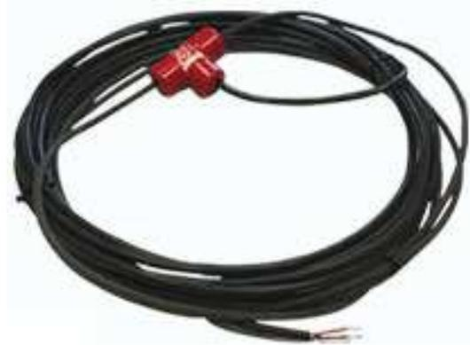
The PFL preformed vehicle detection loop is constructed of stranded wire conductors with XLP thermoplastic elastomer insulation jacketing. The outer shell is flexible nonmetallic 0.26" tubing. The vehicle detection loop includes electronic lightning protection. The lead-in wire is twisted, shielded and 50 ft. long.
