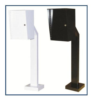
These housings and pedestals are used for the installation of card readers, intercoms and other devices at vehicular and pedestrian access points. Hinged door with cam lock provides both security and ease of access. Standard finish is either white or black powder coat. Model 9050-1-1 includes Model 306-6, 36" tall pedestal and 9050-1BD, 14" H X 9" W housing.
