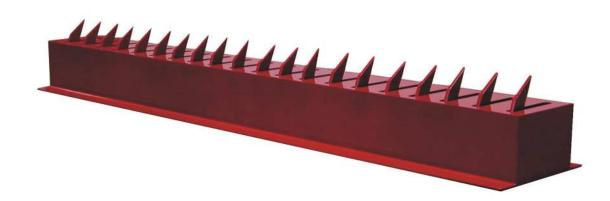
The traffic controller is a heavy duty in-ground "Directional Enforcer". It allows traffic in one direction only. It can be used as a free entrance or exit to your parking facility. It can be used to enforce one-way traffic in such drive-through areas as hotels, banks, commuter stations, etc. The Model 200-1 is 72" wide and includes twenty cut-steel blade teeth.
